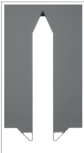
FIG. 2. Optical image of Cantilever 6 in its holding box. The imaging tip (black triangle) is pointing out of the page.
